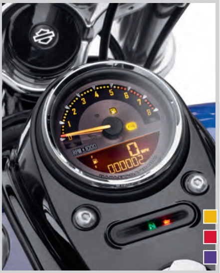
I. DIGITAL SPEEDOMETER/ANALOG TACHOMETER – 4" SPUN ALUMINUM DIAL
